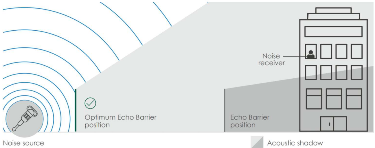
Figure 1 – Barrier Wall Location Placement
